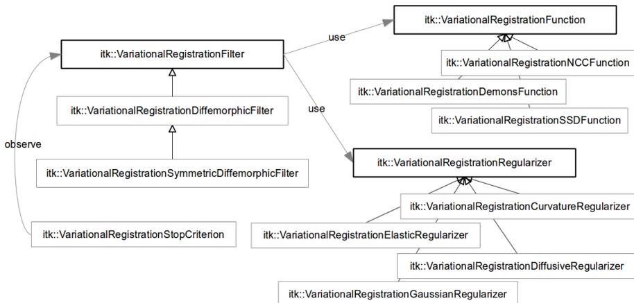
**Fig. 1.** Extraction from the class diagram of the toolbox *VariationalRegistration*. The overall registration algorithm is implemented in the class `VariationalRegistrationFilter` and its child classes for (symmetric) diffeomorphic registration. The force field (related to the distance measure) is computed in child classes of `VariationalRegistrationFunction` and the regularization step is done in classes derived from `VariationalRegistrationRegularizer`.
